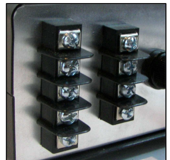
Alarm & RTD Connection
