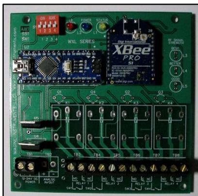
The WXL-ME Series Switch Transmitter features up to 4 dry-contact inputs that activate relays of the receiver unit. The unit also sends supervisory system data to the receiver
