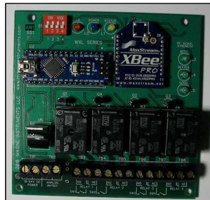
The WXL-ME Series Receiver features up to 4 control relays. The unit also provides an Alarm output for Transmitter low power or RF signal loss.
